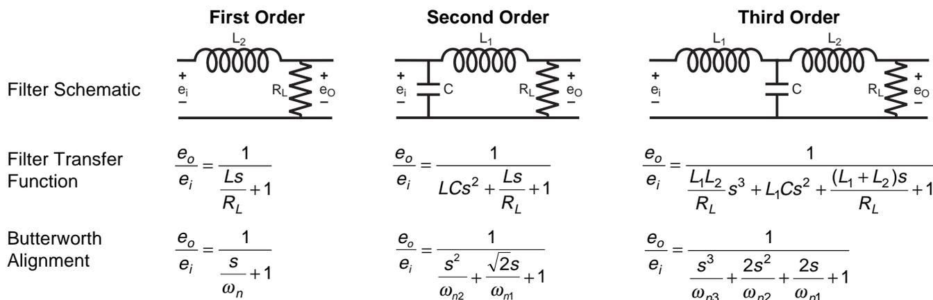
Figure 7 The first three order low pass filters and their Butterworth alignments
