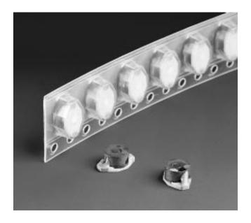
The Coilcraft DT1608 Series represents the ultimate in cost-effective, miniature power inductors. The DT Series is magnetically shielded and the materials used provide natural heat sinking. This allows these parts to be used at relatively large currents. Even at 150% of rated current, the temperature rise is less than 15° C. Because of their "swinging" inductance vs current characteristics, the DT1608 Series can be used as ultra high L inductors at zero or low current.
