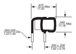
This low cost toroidal inductor is designed for high current, low voltage applications, particularly the latest generation of low voltage microprocessors.
