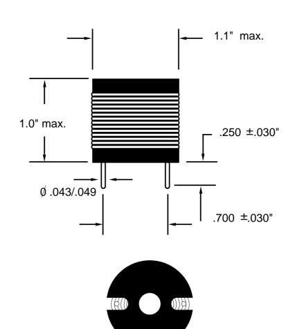
L = 180 uH ± 10% MEASURED ON HP4192A @ 1KHZ/0.1V
