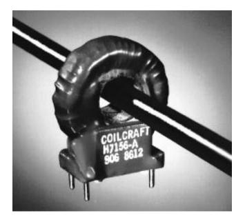
The CS60 Series measures current from 5 to 100 amps RMS. Applications include sensing branch circuit overload and detecting load drop or shutdown. The sensor functions as the encapsulated secondary of a current transformer, while the conductor carrying the current to be measured serves as the "one turn primary." Sensitivity may be enhanced by increasing primary turns.
