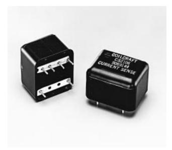
These Coilcraft current sense transformers are intended for use in measuring 50/60 Hz line currents from .5 to 20 Amperes RMS. Typical application as shown below yields a standard output of .1 Volt per Ampere. The sensitivity may be changed easily by simply adjusting the value of the sense resistor. These parts also can be used to measure 400 Hz line currents.
