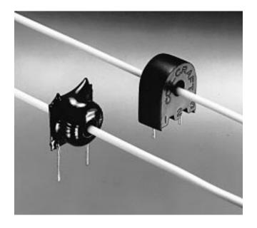
Designed for use at 20kHz-50kHz and higher, these sensors function as the secondaries of a current transformer. The conductor carrying the current to be measured is the "one turn primary." Sensitivity can be set at 1 Volt per Ampere or at other desired values. It can also be doubled by looping the conductor through the hole twice. Applications include sensing branch circuit overload, switcher feedback, and detecting load drop or shutdown.
