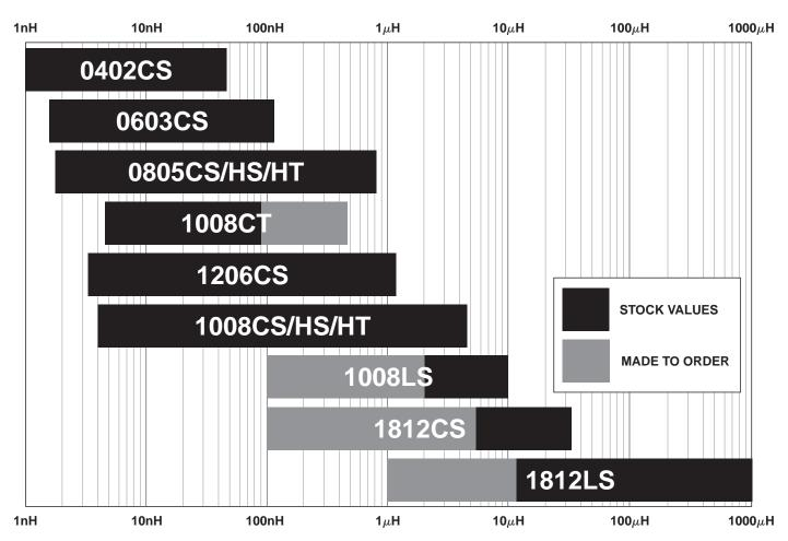
Use this chart to determine which Coilcraft chip inductor family provides the value you need. Follow these tips to select the best overall combination of low cost, close tolerance and high self resonance.
