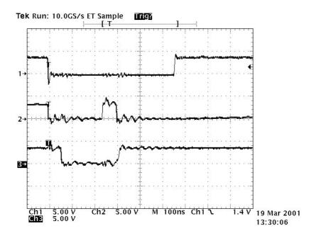
As you can see, the graphic controller is setting its XRDY-line shortly before being ready to HIGH and then when being ready it releases the XRDY-line to LOW (SH3-bus mode). The FR-Microcontroller instead is looking for a HIGH-level after the external device, which is connected to his bus, is ready. So connecting both ready-lines directly together will result in a deadlook after the first READ/WRITE-access.
