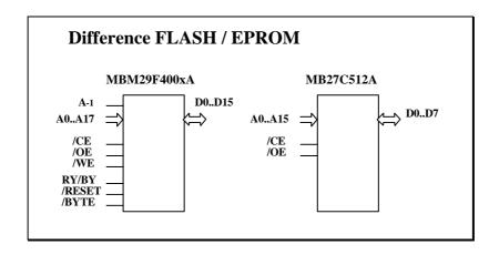
The /BYTE input is used to configure the device to operate in either 8-bit or 16-bit wide mode. If it is configured as an 8-bit memory, the additional address line "A  $_{-1}$ " is needed to address the complete memory area. As mentioned above, for this application note we assume the 16-bit mode, so "A  $_{-1}$ " is not used.
