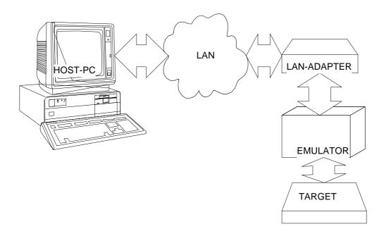
The Fujitsu emulators MB2141 and MB2197-01 respectively for the 16bits- and the FR-flash-microcontroller are provided with a local area network adapter that can be used to programme and debug a device over a network connection. No additional hardware connection except the LAN connection is required for this purpose
