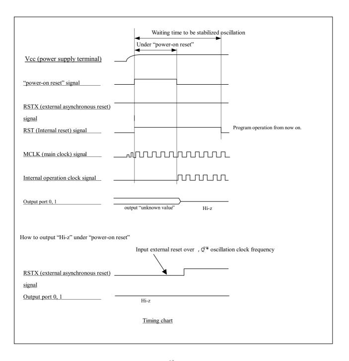
Under "power-on reset"  $2^{17}$  \* oscillation clock frequency (8.192ms in case of oscillation clock frequency = 16MHz)
