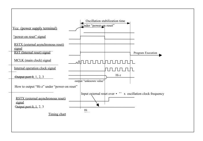
Under "power-on reset"  $2^{17}$  x oscillation clock frequency (8.192ms in case of oscillation clock frequency = 16MHz)
