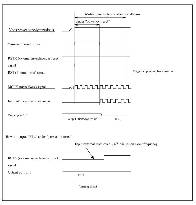
Under "power-on reset" • \* oscillation clock frequency (8.192ms in case of oscillation clock frequency = 16MHz)
