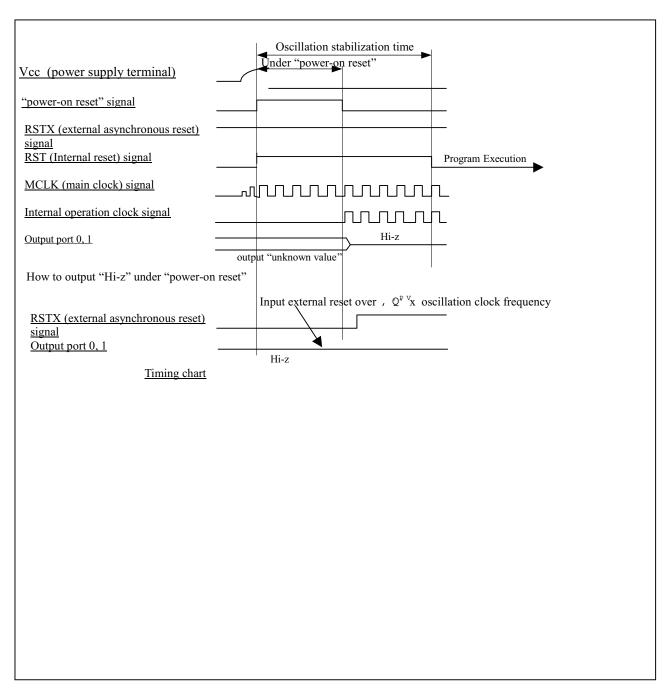
Under "power-on reset"  $\Box^{\square\square}$  x oscillation clock frequency (8.192ms in case of oscillation clock frequency = 16MHz)
