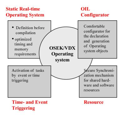
Defined as a highly scalable operating system some features may be switched off. In order to obtain interoperability, different sets of features are defined as "conformance classes". osCAN supports all conformance classes.
