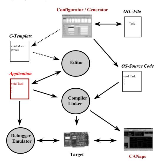
**Debugging** is performed as usually. Vector Informatik offers with **CANape** a powerful tool to monitor the target system via the CAN-bus online but remote. This allows a debugging in standard operating conditions when an emulator is no more applicable.
