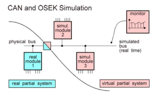
**I/O interfaces** of the hardware may be simulated completely by CANoe. I.e. outputs are displayed and inputs are processed. This is achieved by the generic interface offered by the environment variables of CANoe. The user has to implement only an abstraction layer. This layer will be replaced by the specific I/O access when porting to the target hardware. The maximum count of environment variables, i.e. I/O channels, is almost unlimited.
