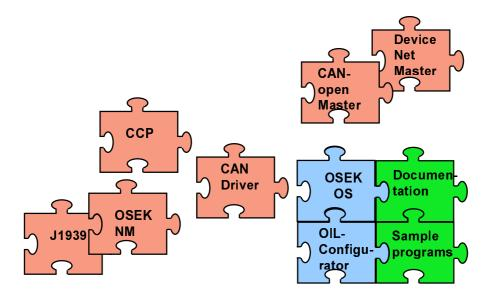
For industrial purposes the widely used **CANopen** and **DeviceNet** protocol stacks may be chosen. Automotive applications are provided with the complete set of software modules like CAN-driver, network management, transport protocol, Can Calibration Protocol etc.
