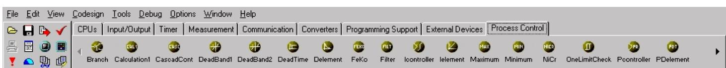
**Process Control beans** are Embedded Beans™ that implement a wide range of function modules for industrial applications. Most of them are designed for closed loop controlling, but many beans for standard control applications are also included. Like all other beans, they have properties, methods and events.
