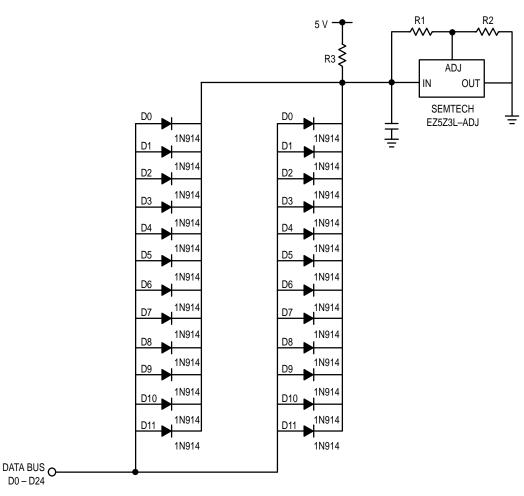
Figure 5. 5 V to 3.3 V Regulator Circuit
