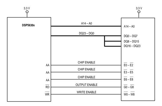
Figure 3. DSP5630x Connection to (32K x 8) Based Module on X, Y, and P Memory
