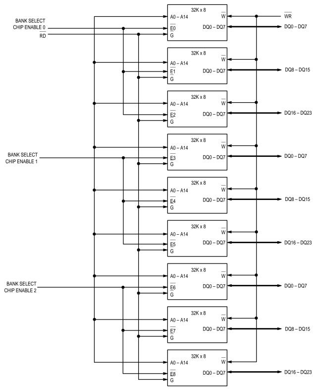
NOTE: The chip enables are connected to the AA pins of the DSP.
