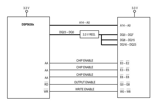
Figure 4. DSP5630x Connection to (32K x 8) Based Module on X, Y, or P Memory
