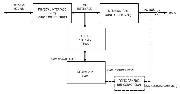
NOTE: The FPGA uses several signals of both the CAM, MAC, and PHY.
