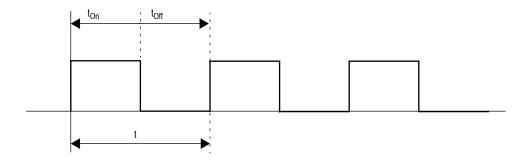
Figure 1. PWM Signal with 50% Duty Cycle
