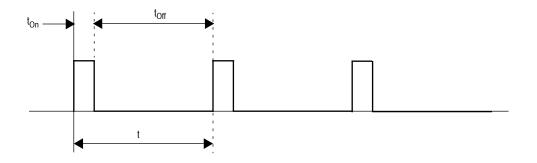
Figure 2. PWM Signal with 10% Duty Cycle
