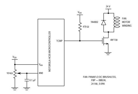
Figure 4. Fan Control Circuit
