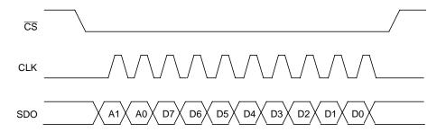
Figure 3. Serial Data Timing
