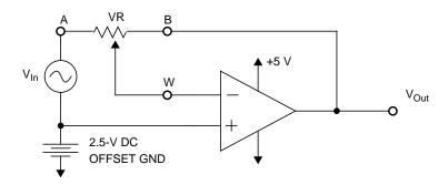
Figure 7. Programmable Inverting Op Amp
