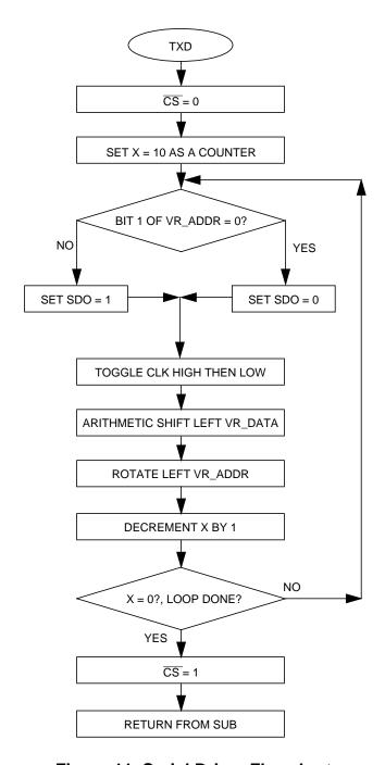
Figure 11. Serial Driver Flowchart
