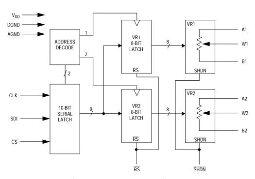
Figure 2. AD8402 Block Diagram
