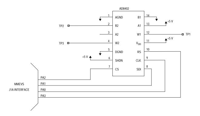
Figure 10. J1A to AD8402 Interface Test Circuit
