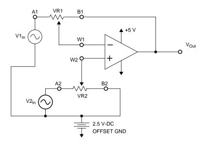
Figure 9. Programmable Differential Op Amp
