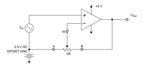
Figure 8. Programmable Non-Inverting Op Amp
