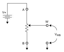
Figure 6. Programmable Potentiometer Divider
