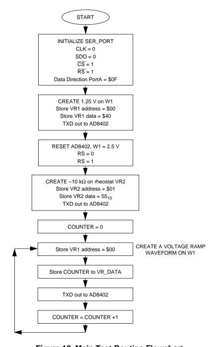
Figure 12. Main Test Routine Flowchart
