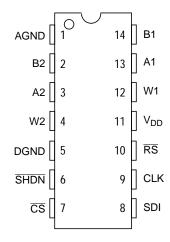
Figure 1. AD8402 Pinout
