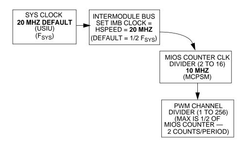
Figure 4. PWM Clock Arrangement
