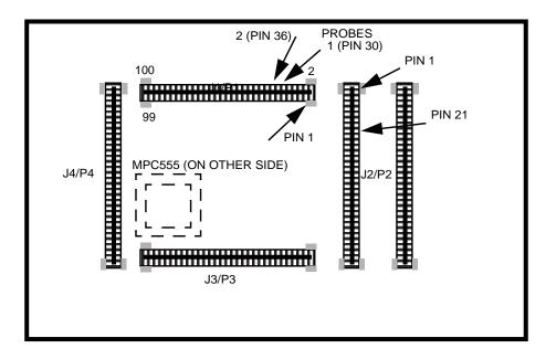
Figure 3. Underside of MPC555 EVB
