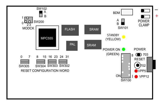
Figure 1. Evaluation Board Layout
