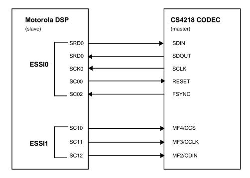
Figure 2. ESSI/CODEC Pin Setup
