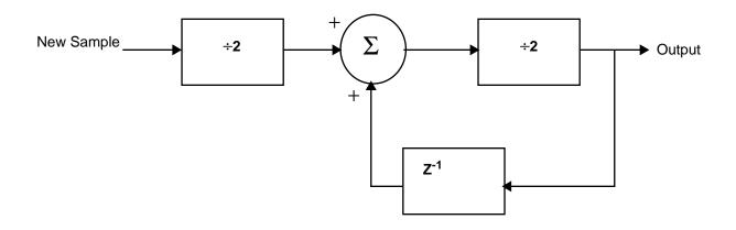
Figure 3. Block Diagram of a Delayed Sample (Echo)
