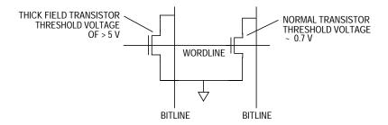
Figure 6. Bitcell Schematic Diagram
