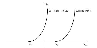
Figure 9. Effects of Programming and the V<sub>T</sub> of a Bitcell
