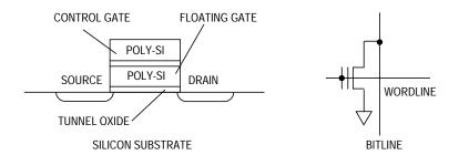
Figure 16. 1T FLASH Bitcell Cross Section and Schematic
