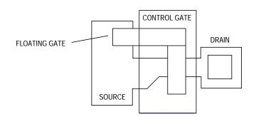
Figure 14. 1.5T FLASH Bitcell Top Down View
