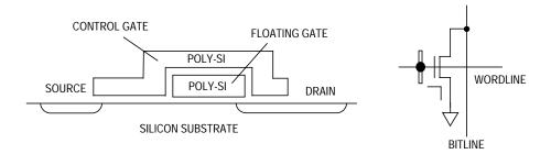
Figure 13. 1.5T FLASH Bitcell Cross Section and Schematic
