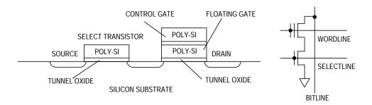
Figure 15. 2T FLASH Cross Section and Schematic
