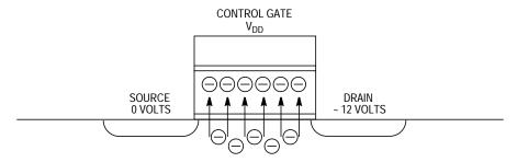
Figure 8. Channel Hot Electron Programming Mechanism
