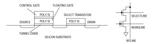
Figure 10. EEPROM Bitcell Cross Section and Schematic
