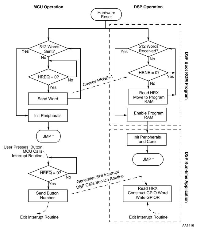
Figure 2-2 DSP-MCU System Flow Diagram
