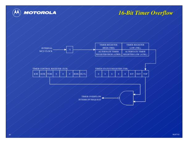
All functions of the 16-bit timer are related to the 16-bit counter which serves as its time base.
