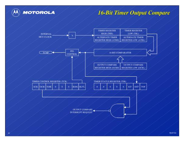
Output compare is essentially a method for generating delays, because it allows future events to be synchronized to the current value of the 16-bit timer counter.
