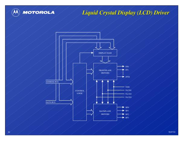
All 68HC05 "L" family members have liquid crystal display (LCD) interfaces of varying degrees of sophistication. A representative implementation is the LCD driver on the popular MC68HC705L16, shown in the block diagram above.
