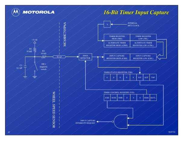
Input capture functions like output compare in reverse. Instead of generating an edge on the TCMP pin at a specific time, input capture saves the time at which a specific edge occurs on the TCAP pin.
