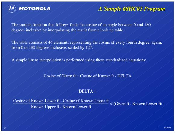
To simplify the interpolation math, the look up table includes the cosine of every fourth degree  $(0^{\circ}, 4^{\circ}, 8^{\circ}, \text{ and so on})$  rather than, say, every fifth degree  $(0^{\circ}, 5^{\circ}, 10^{\circ}, \text{ and so on})$ .
