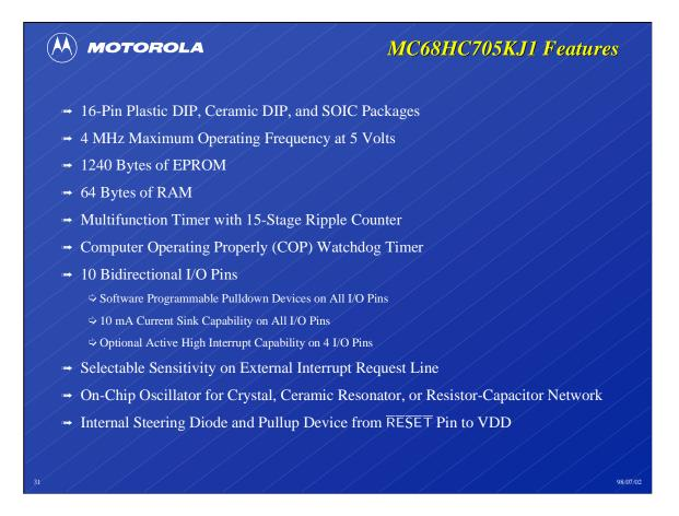
For it to be an affordable replacement for conventional dimmers, the smart light dimmer needs a cost-efficient microcontroller. The MC68HC705KJ1 fits the bill by providing features appropriate for this application.
