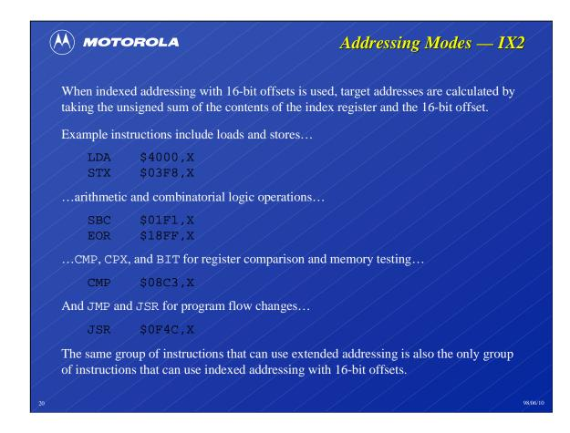
Instructions that use indexed addressing with 16-bit offsets can read from or write to any location in the 68HC05 memory map. These instructions always require three bytes of storage.
