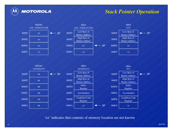
Processor state is saved on the stack when changes in program flow occur. The 68HC05 has a 64-byte hardware-controlled stack. Reset initializes the stack pointer to \$00FF; the RSP instruction does the same. No other instructions allow direct user manipulation of the stack.
