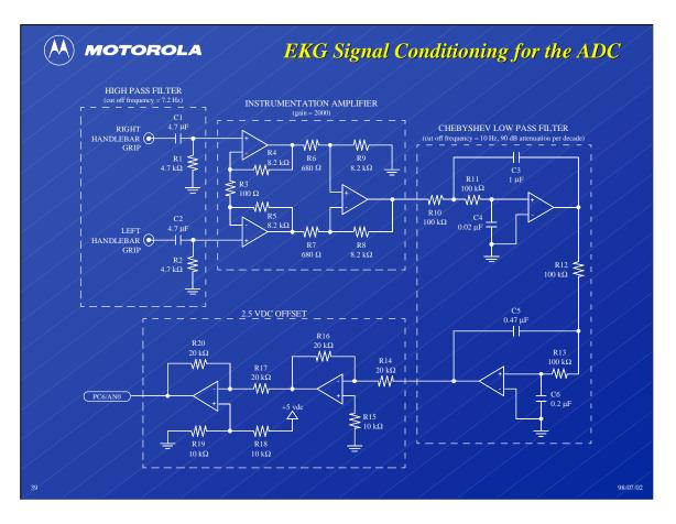
The cycling computer uses the analog-to-digital converter to sample the EKG signal that appears across the handlebar contacts when they are gripped.
