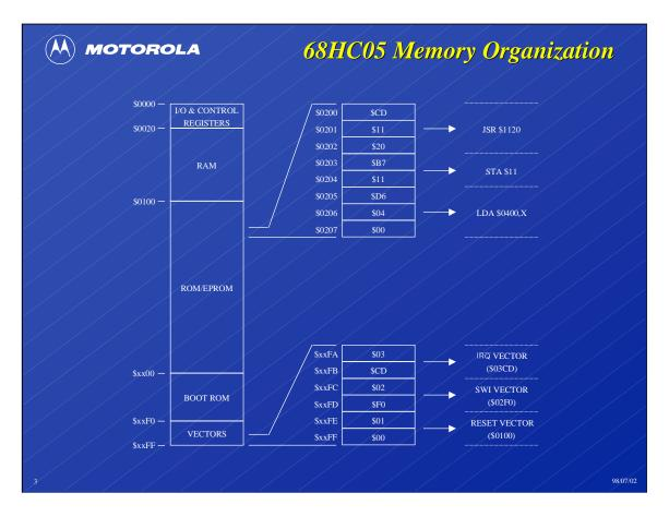
The 68HC05 is a Von Neumann computer. All storage and input/output resources are memory mapped into a single linear address space.
