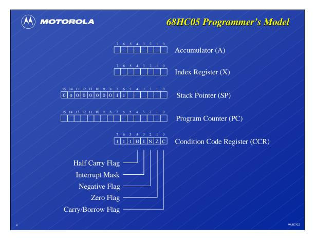
The 68HC05 central processor unit (CPU) consists of an accumulator (A), an index register (X), a stack pointer (SP), a program counter (PC), and a condition code register (CCR).
