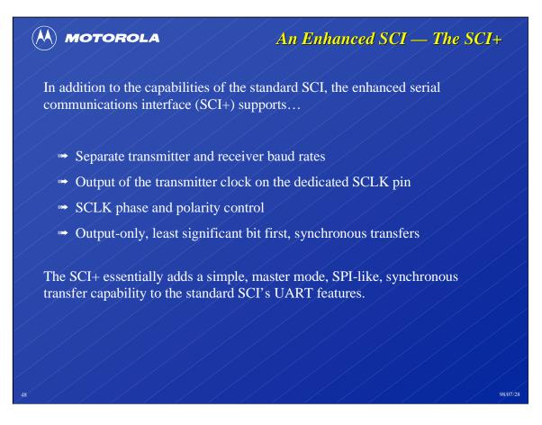
As noted above, the SCI+ can perform simple, output-only, synchronous transmissions in addition to its standard UART functions.
