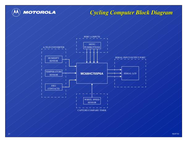
For riders to find the cycling computer useful, it must collect and present its statistics with a minimum of fuss. Ambient temperature and humidity are easily monitored with sensors attached to the cycling computer's housing, but the rider's heart rate presents a special problem.
