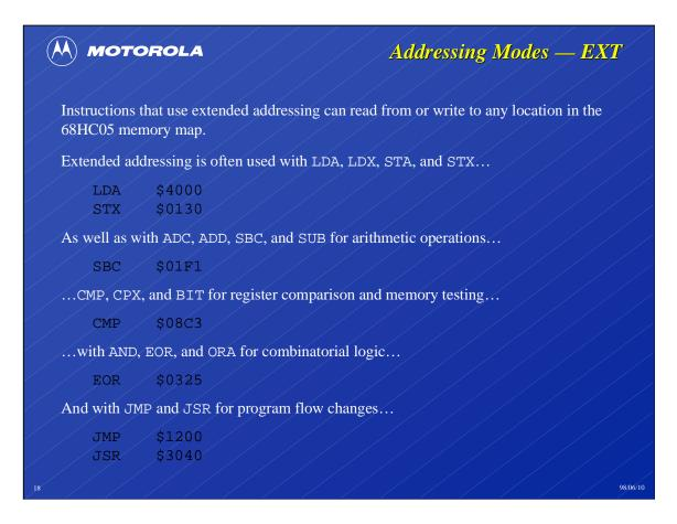
Extended addressing allows any location in the 68HC05 memory map to be read from or written to using a single instruction. The address is always specified using a 16-bit value.
