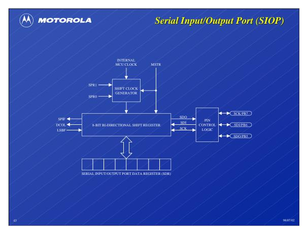
The serial input/output port (SIOP) is a simplified version of the serial peripheral interface (SPI) that appears on numerous Motorola microcontrollers ranging from other 68HC05 devices to members of the highly-integrated 68300 family. The SIOP supports master (processor initiated) and slave (externally initiated) mode transfers.
