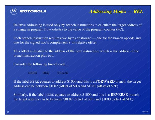
Only branch instructions use relative addressing. A branch instruction executes in three clock cycles and consists of two bytes. The first byte is the opcode for the particular branch condition, and the second byte is a signed two's complement offset from the address of the next instruction.
