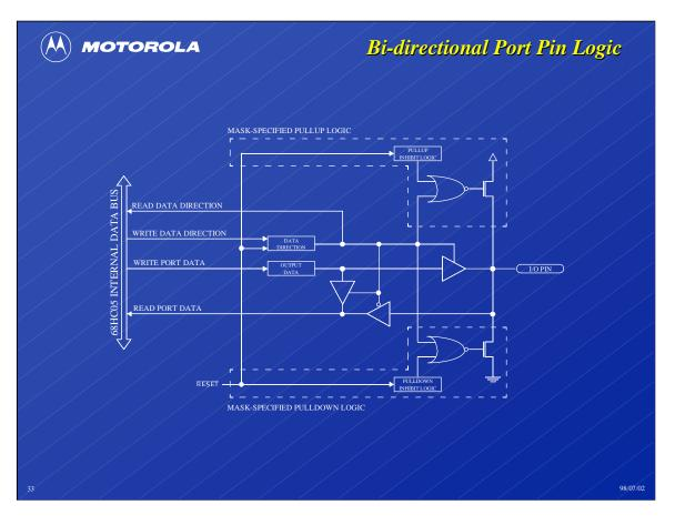
The diagram above shows a simplified version of the logic that comprises a bidirectional port pin. I/O pins, typically in groups of eight, comprise a single port.
