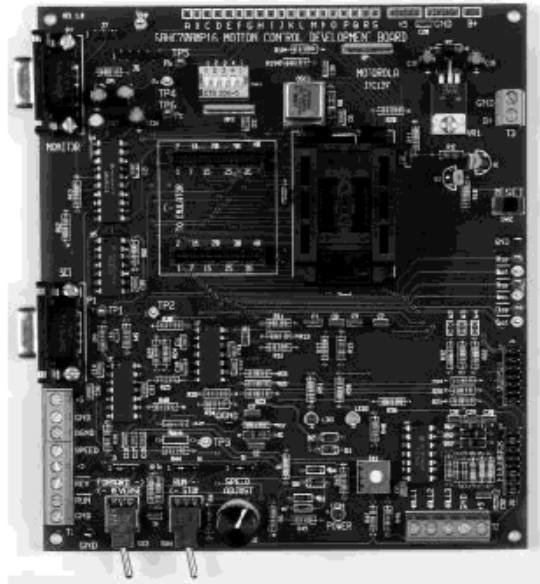
Figure 1. ITC137 Development Board
