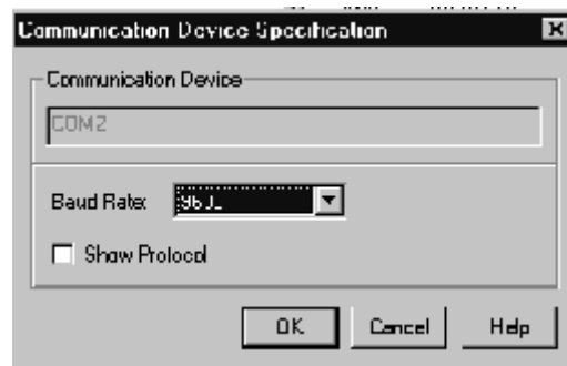
Figure 2-24. Communication Device Specification Dialog
