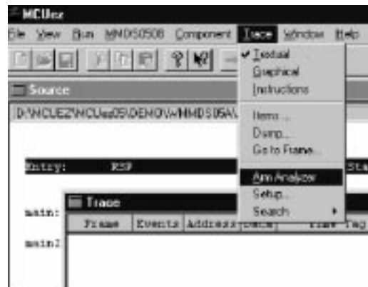
Figure 2-32. Selecting Arm Analyzer From Trace Menu
