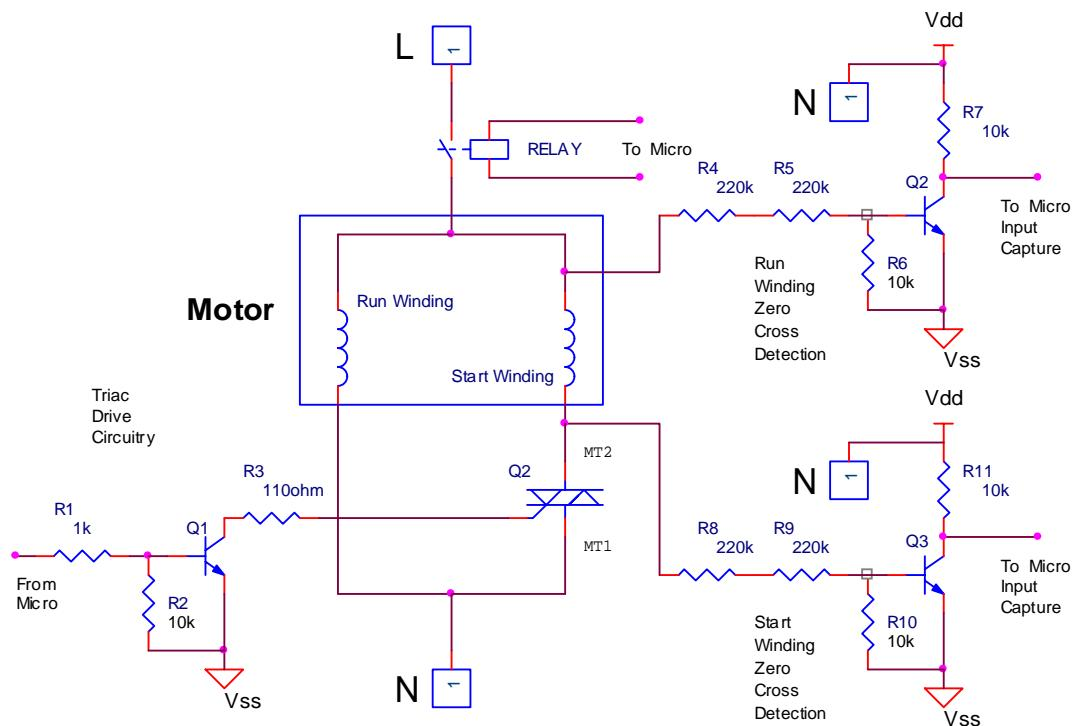
When running, the continuous rotational motion of the motor and magnetic field induces a voltage in the now redundant start winding. During normal running conditions there is a measurable phase difference between the start and run windings. This is illustrated in the following diagrams.
