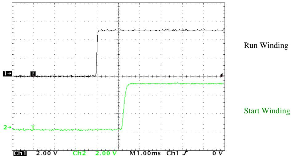
This is the digital representation of the phase difference between the run and start windings during normal running conditions.
