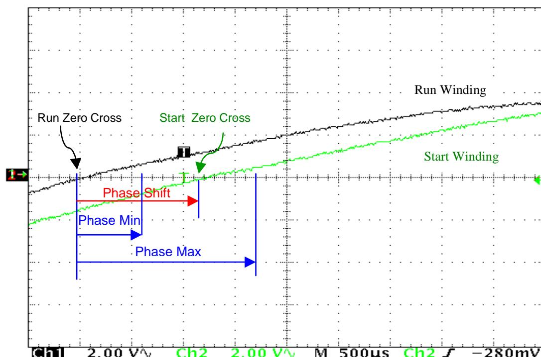
The 'phase shift' is the actual phase difference between the run and start windings. 'phase min' and 'phase max' define the acceptable tolerance band for the detection of the start zero cross point from the run zero cross reference point.
