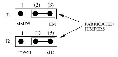
Jumper J2 can be used to select between an internal generated clock or a external clock generated by the target system. If the target clock is selected by placing the jumper on J2 between pins 1 and 2 the position of the fabricated jumper on J1 does not matter.
