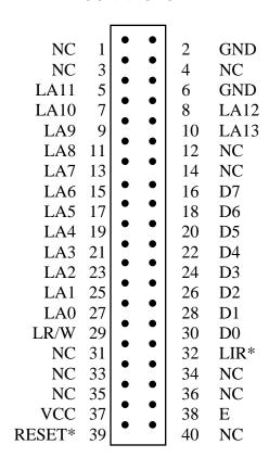
Figure 3-1. Connector P1 Pin Assignments
