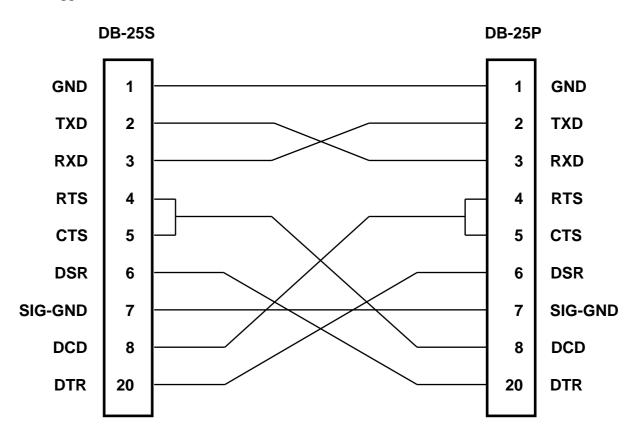
FIGURE 4-2 Null Modem Adapter
