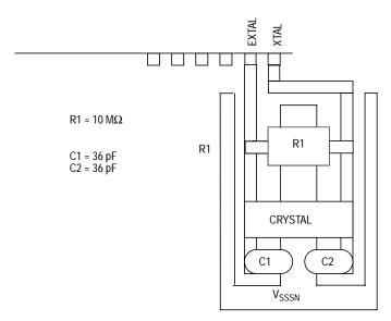
Figure 3. Suggested Crystal Oscillator Layout
