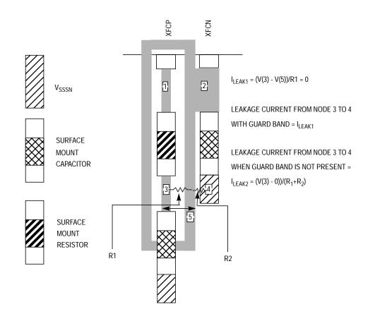
Figure 2. Guard Banding to Reduce Leakage
