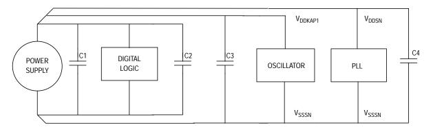
Figure 6. Star Point Power Supply Connection
