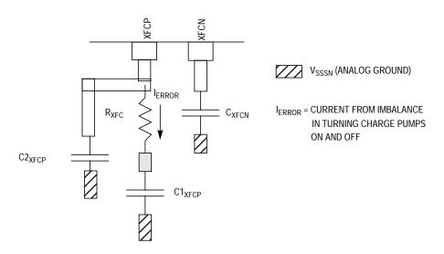
Figure 4. Bypass Capacitor (C2<sub>XFCP</sub>) for Improved Jitter Performance
