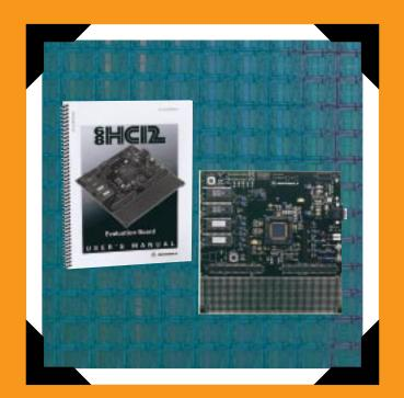
ardware and software designs based on the 68HC12 architecture can be evaluated and debugged quickly and efficiently with Motorola's full-featured evaluation board.
