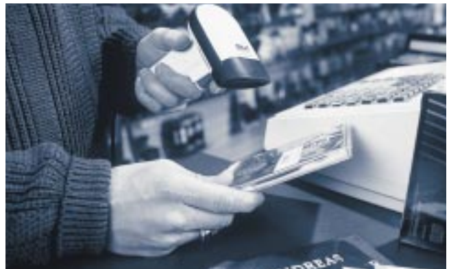
THE 68HC16Z1, WITH ON-CHIP DSP CAPABILITIES, POWERS SPECTRAPHYSICS' HAND-HELD BARCODE SCANNER.
