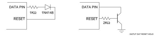
Figure 2 Alternate Methods of Conditioning Data Bus Pins
