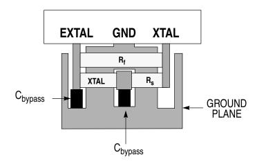
Figure 5 Typical One-Layer Oscillator Layout
