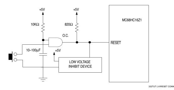
Figure 7 Typical MC68HC16Z1 Reset Circuit
