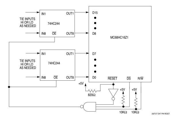
Figure 1 Circuitry to Drive Data Bus Pins During RESET Assertion
