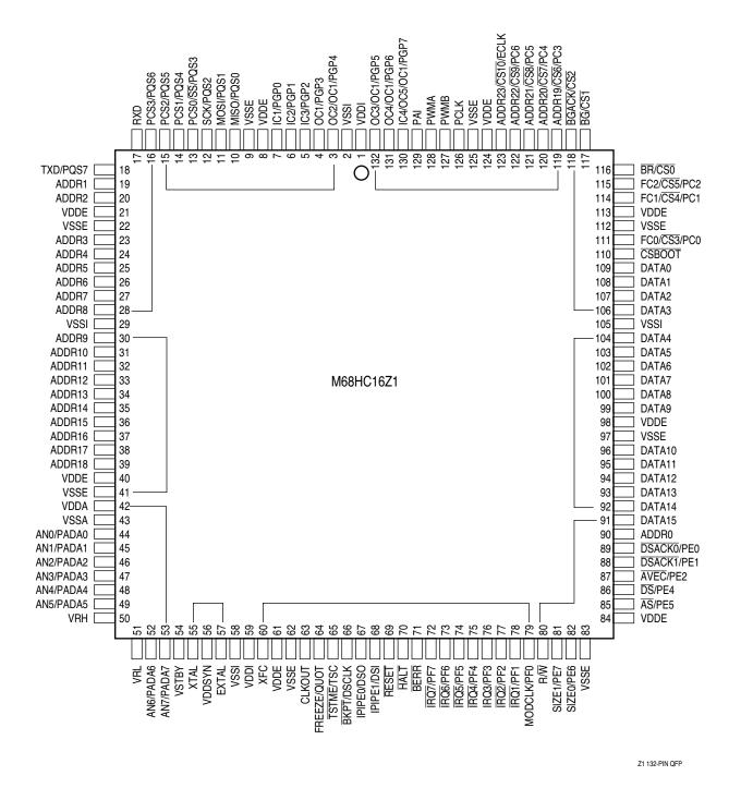
Figure 10 Pinout of MC68HC16Z1 132-Pin Package
