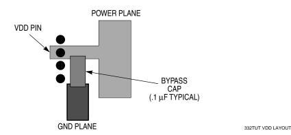
Figure 11 Proper Placement of a Bypass Capacitor
