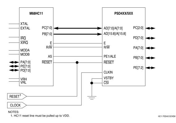
Figure 2 Typical M68HC11 and PSD4XX/5XX System
