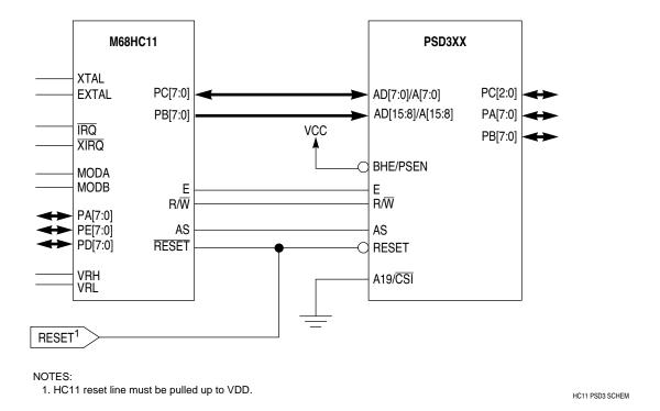
Figure 1 Typical M68HC11 and PSD3XX System
