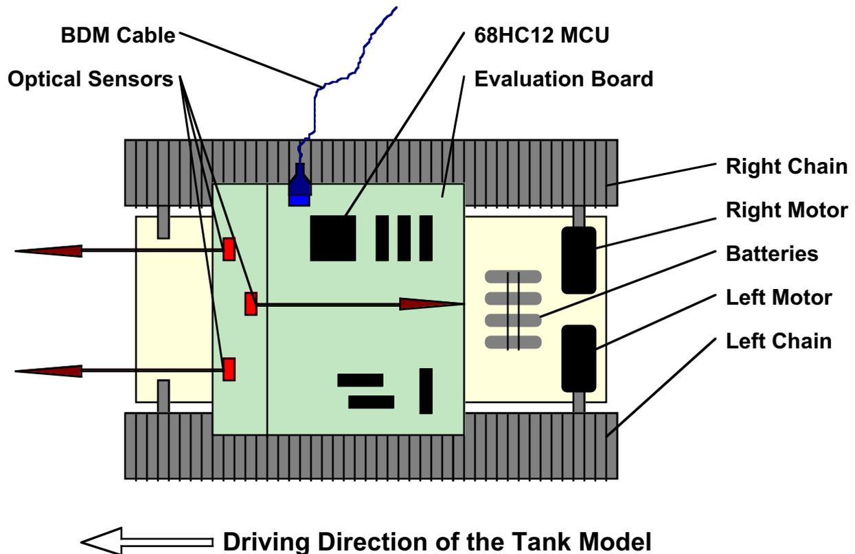
Figure 2 Scheme of the Tank Demonstration Model
