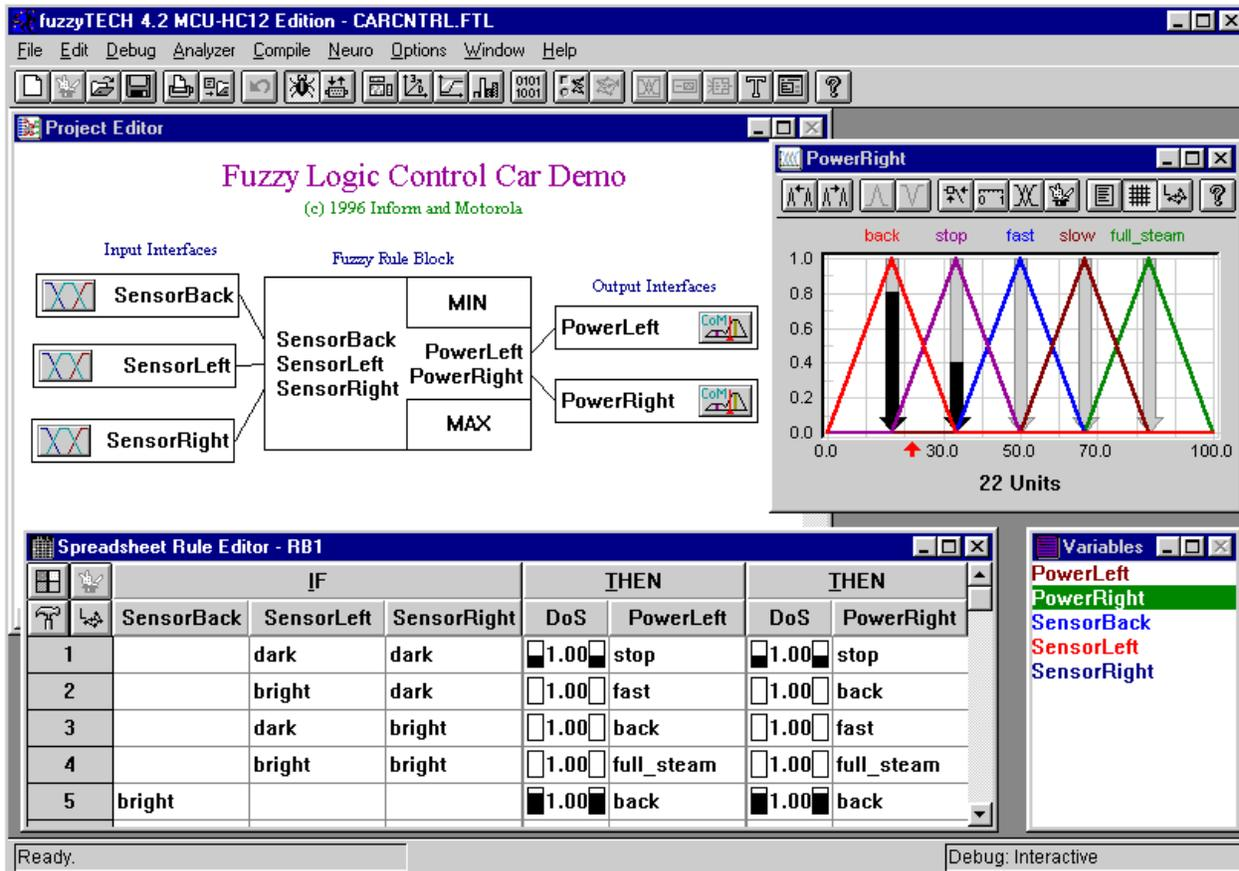
Figure 3 Fuzzy Logic Controller Development Using *fuzzyTECH*
