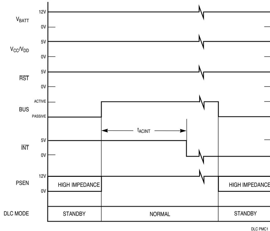
**Figure 2-4 Method 1 — Standby Mode Supplies Applied**
