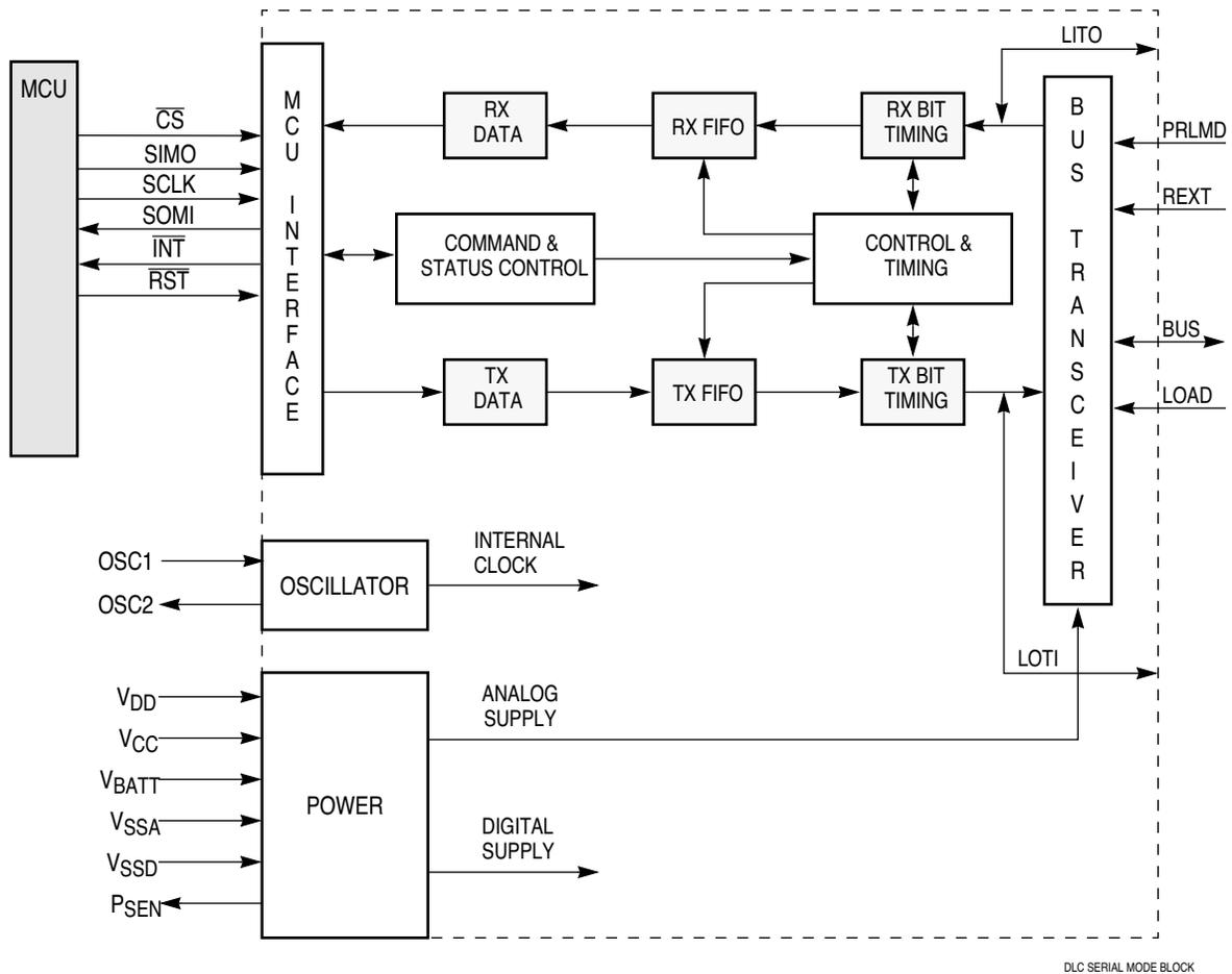
**Figure 1-2 MC68HC58 DLC Serial Mode Block Diagram**
