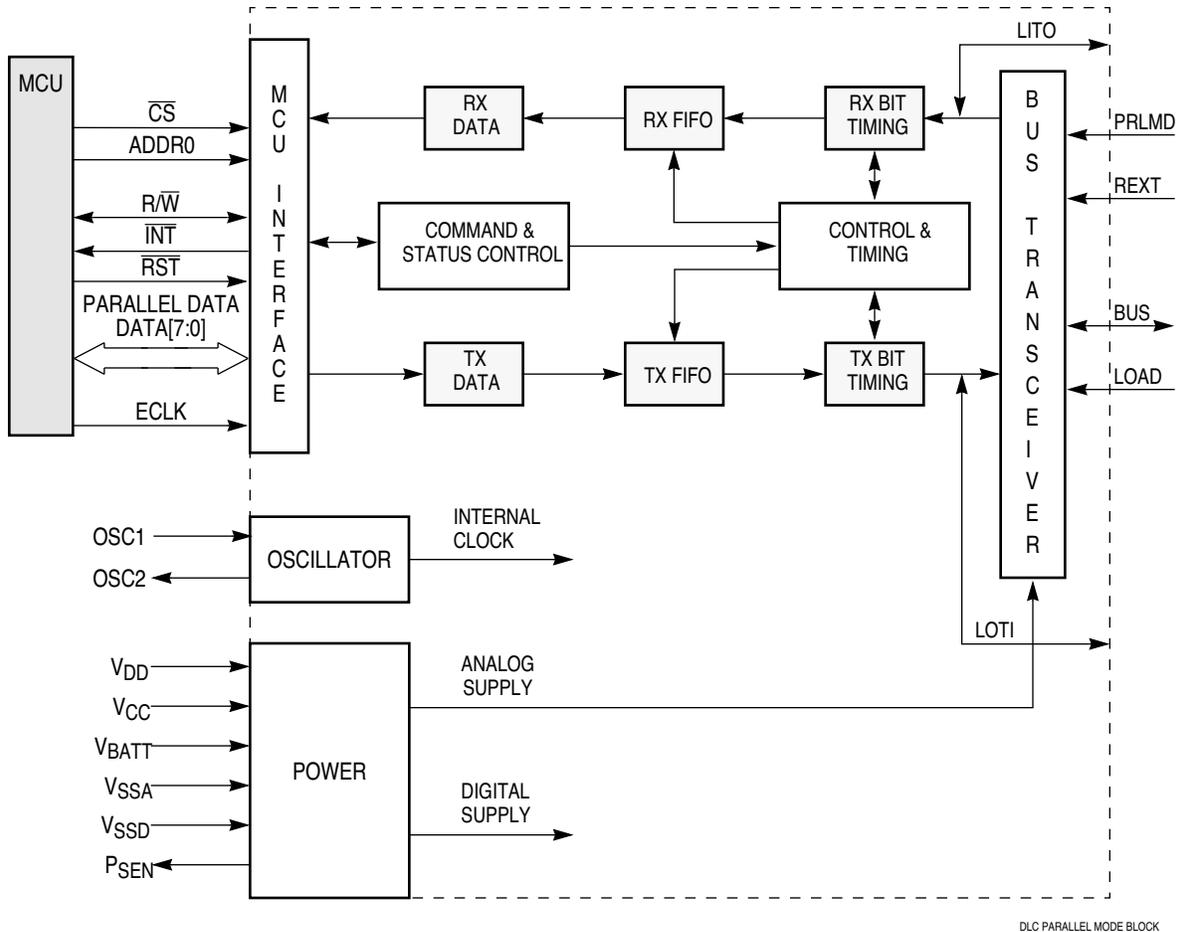
**Figure 1-1 MC68HC58 DLC Parallel Mode Block Diagram**
