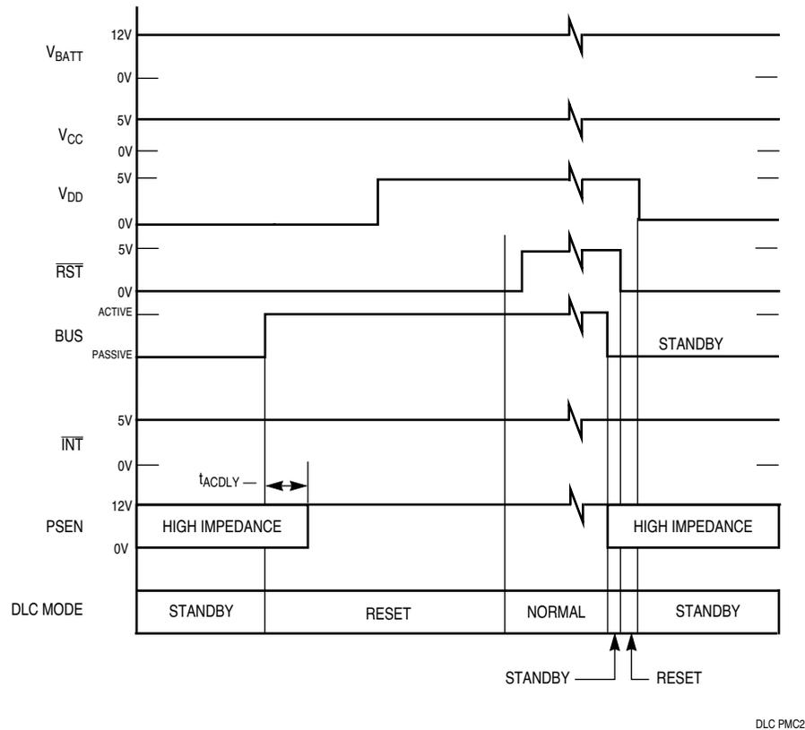
**Figure 2-5 Method 2 — Switching  $V_{DD}$  with PSEN**
