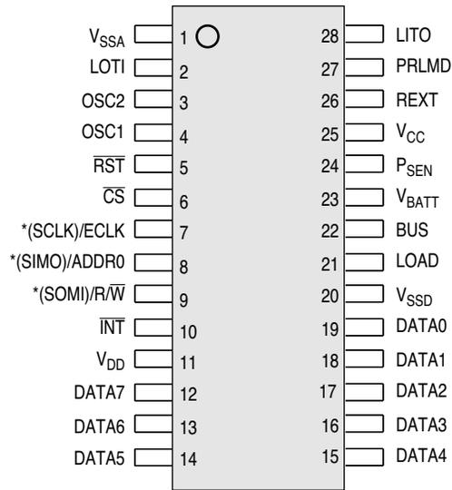
\* ( ) INDICATES PIN ASSIGNMENTS FOR SERIAL MODE OPERATION
