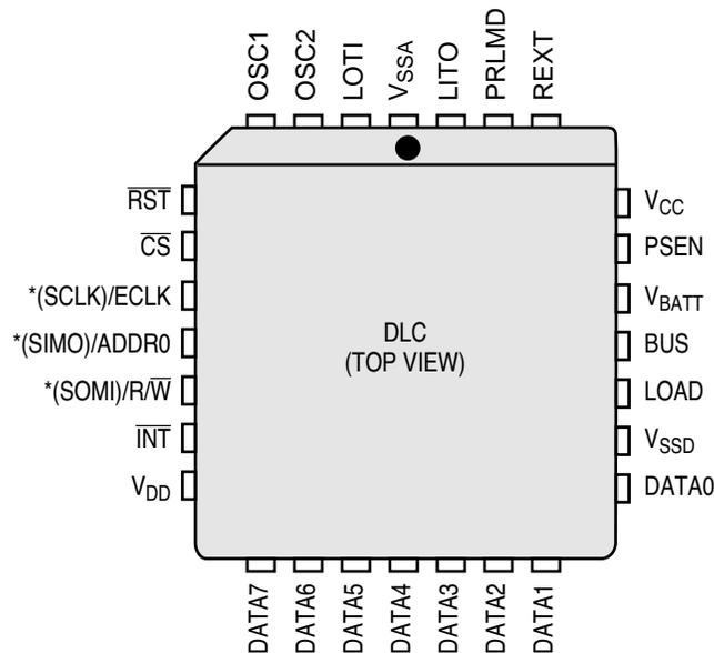
\* () INDICATES PIN ASSIGNMENTS FOR SERIAL MODE OPERATION
