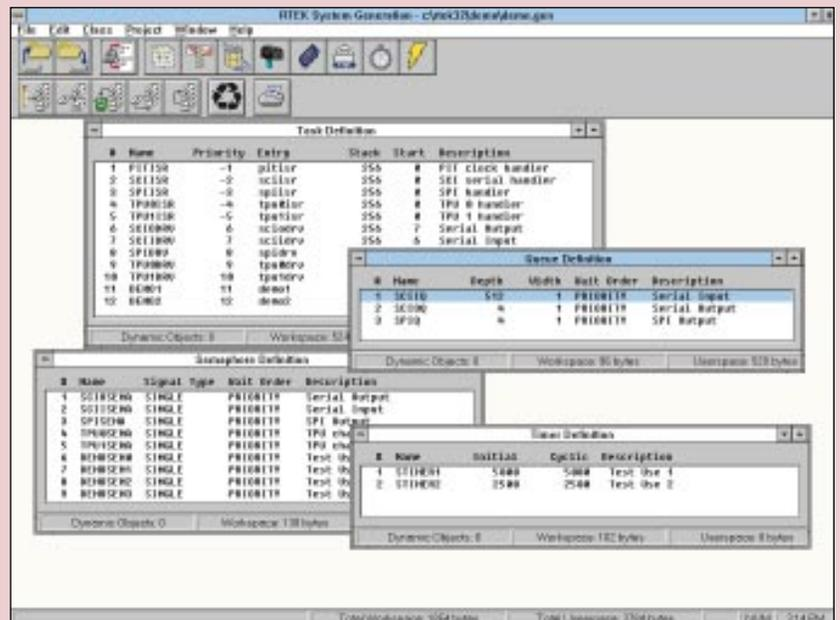
RTEKgen allows easy system configuration by giving designers a simple way to define the system architecture.
