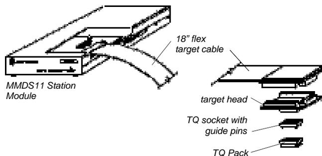
**Note:** The following device-specific components must be purchased separately from the station module. An emulator module, target head or flex cable can often be adapted to a wide range of M68HC11 devices. Consult the table on page 26 to order the appropriate MMDS11 system.
