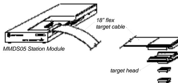
**Note:** The following device-specific components must be purchased separately, according to the specific MCU device in use. An emulator module or a target cabling component can be used for multiple devices in the M68HC05 and M68HC08 families. Consult the table on page 15 to order a complete MMDS system.
