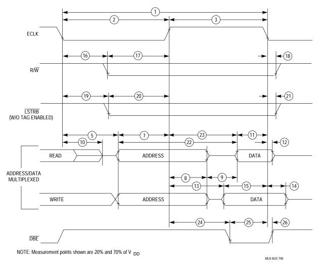
Figure 8 Multiplexed Expansion Bus Timing Diagram
