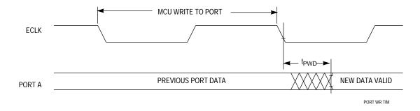
**Figure 7 Port Write Timing Diagram**
