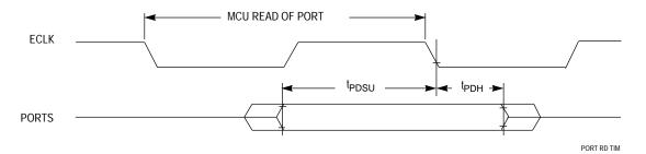
**Figure 6 Port Read Timing Diagram**
