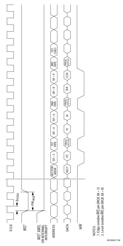
**Figure 5 Interrupt Timing Diagram**
