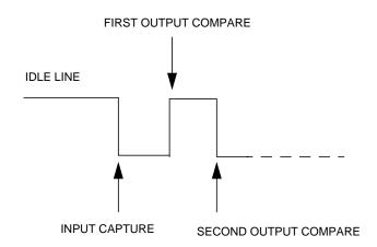
Figure 4. Receiving with the Timer Functions
