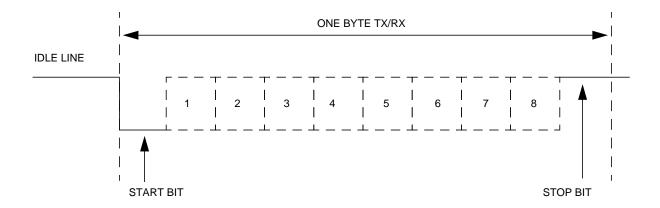
Figure 1. Serial RS-232 Timing
