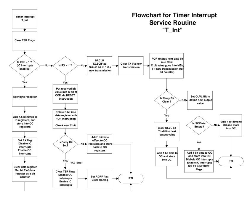
Figure 6. Flowchart for Timer Interrupt Service
