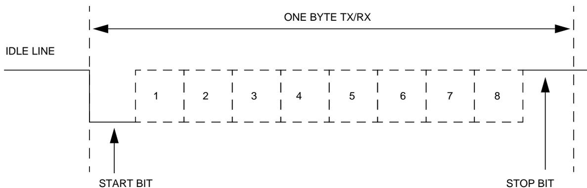
**Figure 1. Serial RS-232 Timing**
