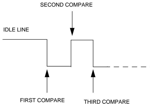
**Figure 5. Transmitting with the Output Compare Function**
