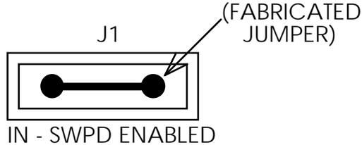
Alternatively, you may use these pins as regular Port A or B pins. To do so, remove the jumper from header J1.
