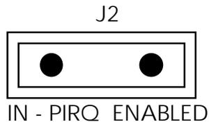
Alternatively, you may OR the PA0-PA3 pins with the IRQ signal to produce IRQ interrupts. For this arrangement, insert a fabricated jumper into header J2.
