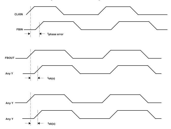
Figure 2. Phase Error and Skew Calculations
