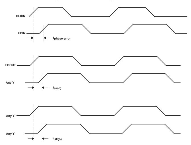
Figure 2. Phase Error and Skew Calculations
