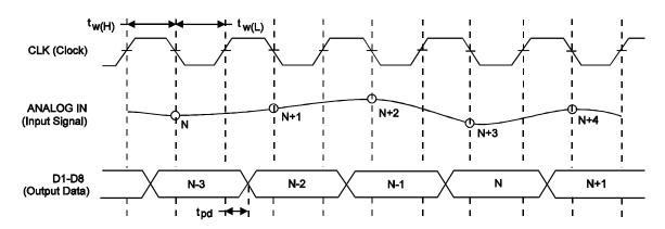
The digital data is valid after a delay time  $t_{pd} = 30$  ns for the TLC5510. Table 1 summarizes important TLC5510 parameters.
