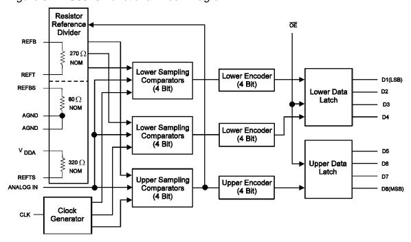
Figure 3. TLC5510 Functional Block Diagram
