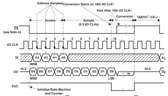
NOTE A: To minimize errors caused by noise at  $\overline{CS}$ , the internal circuitry waits for a setup time after  $\overline{CS}\downarrow$  before responding to control input signals. No attempt should be made to clock in input data until the minimum  $\overline{CS}$  setup time has elapsed.
