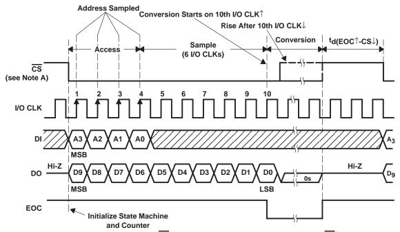
Figure 4–2. Microprocessor Interface Timing (Normal Sample Mode, INV CLK = High)
