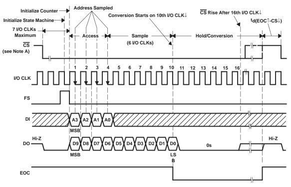
NOTE A: To minimize errors caused by noise at  $\overline{CS}$ , the internal circuitry waits for a setup time after  $\overline{CS}\downarrow$  before responding to control input signals. No attempt should be made to clock in input data until the minimum  $\overline{CS}$  setup time elapses.
