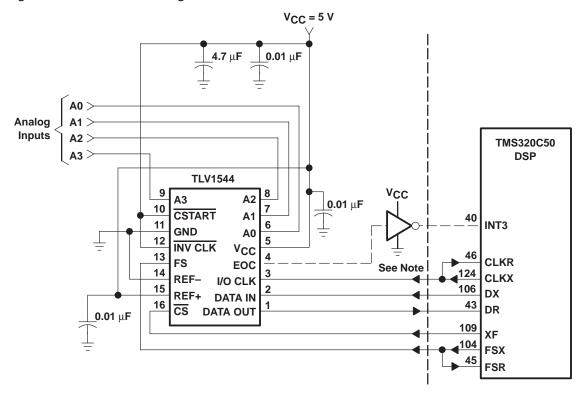
NOTE: Software programs using interrupt processing may need the inverter and the connection shown in dotted lines. In programs using wait states, EOC is not required.
