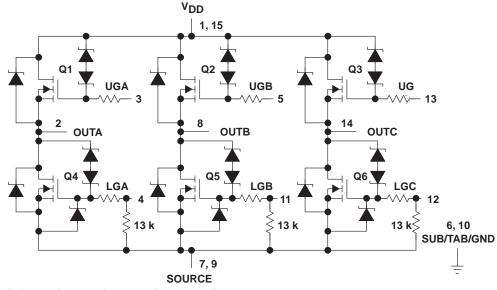
NOTES: A. Terminals 1 and 15 must be externally connected.
