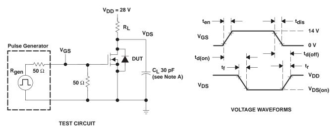
NOTE A: CL includes probe and jig capacitance.
