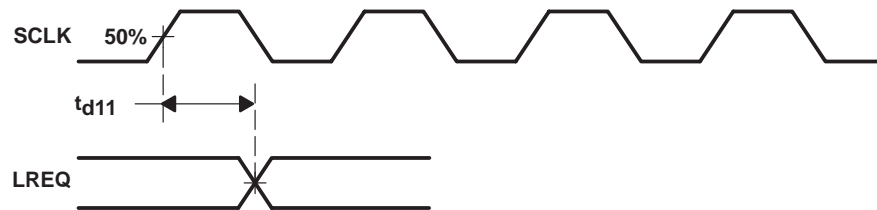
Figure 6-7. TSB12C01A Link-Request-to-Phy-Layer Waveforms
